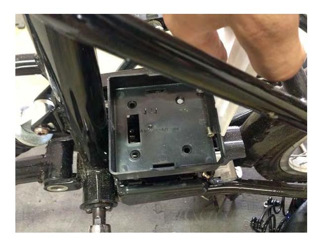
Picture of battery guide rail/battery seat removed:
