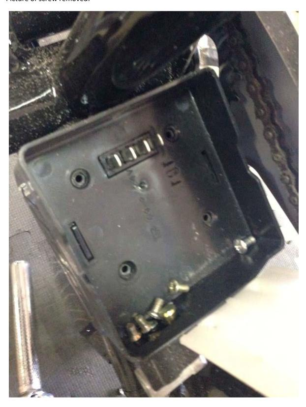
Now you can remove the battery guide rail and battery seat (all one unit):
